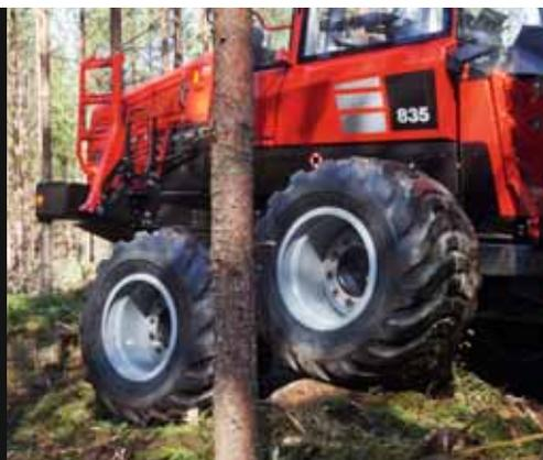
The 835 has a new weight-optimised frame system that in combination with the option of having extra-wide tracks, produces minimal impact on the forest floor. The smooth, V-shaped frame provides outstanding obstacle clearance and manoeuvrability.
