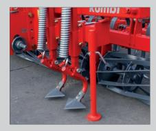
**Tractor track openers** with adjustable working depth.
