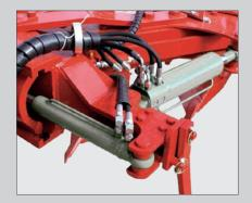
**Hydraulic cylinders**to adjust the plowing width and set of first furrow. The plough can be conveniently controlled from the tractor cabin.
