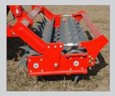
A double reverse-action spike roller provides double-layer cultivation of topsoil.
