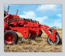
**PLOW in S version**has got Non Stop spring-leaves protection of tines.
