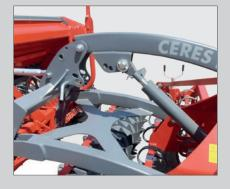
**Solid seed drill coupling** to form combined cultivator and a seed drill unit.
