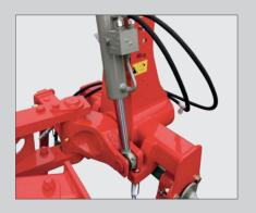
**Swivel axis** with bearing and bi-directional cylinder..
