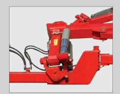
**Rigid head** and easy turning system are the advantages of two hydraulic cylinders of large diameter of Weber Hydaulik production.
