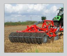
**CROSS 3 S with Drive system** with tyre roller ø670 and disc harrow of B type.
