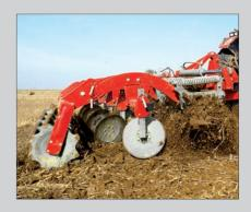
**B-type harrow** two-row ground following and soil mixing harrow of B-type with an adjustable working depth.
