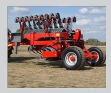
**Transport position** of the TERIS machine ensures safe transportation of the roller on public roads.
