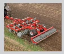
**System LONG**An additional row of tines with a narrow coulter provides greater aeration of soil up to 20 cm.
