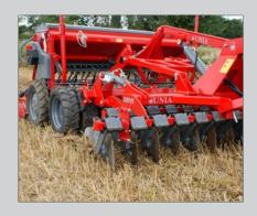
**Drive System**The unit equipped with a tyre roller, which enables transport on roads, soil levelling, clod crushing and soil compaction in strips.
