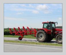
**Plough in transport position** equipped with side support and transport wheel
