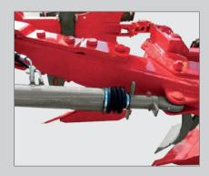
**Cylinder of frame leaning (optional)** relieves the hydraulic system while turning and improves transport on public roads.
