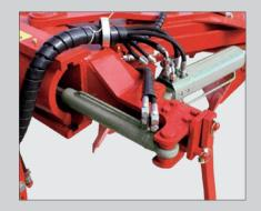
**Hydraulic adjustment** (optional) of the first body provides comfortable work.
