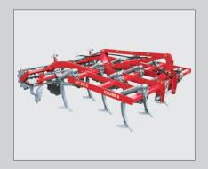
**CROSS S** mounted version with spring protection of tines.
