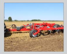
**Set of CX tines** and a spatial frame design ensure reliable operation without stucking.
