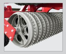
**Cambridge roller** of rings diameter alternatively 525/530 mm
