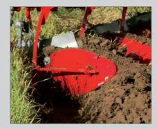
The design of the body allows to position a wide furrow, while minimizing resistance and power requirements of tractors.
