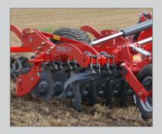
**Large diameter and shape of disc** enables aggressive cultivation and mixing of soil with large amounts of crop residues.
