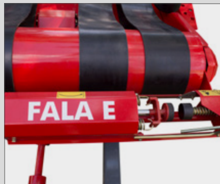
Blade cuts off the film and holds it for next wrapping
