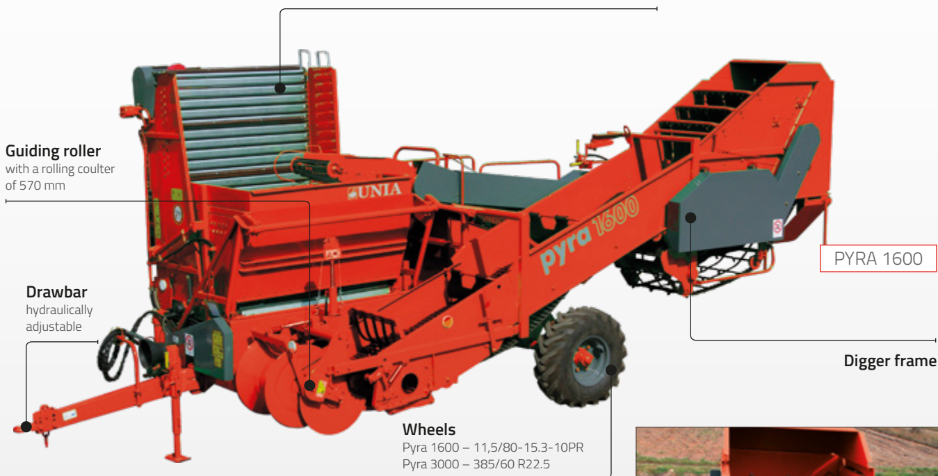
Potato hopper Potato load capacity 1600 kg (Pyra 1600) or 3000 kg (Pyra 3000) Unloading height 1.35 – 2.70 (Pyra 1600)
