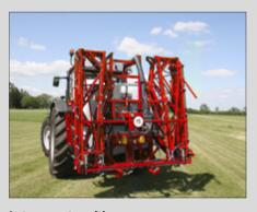
In transport position the width is only 2.55 m, which ensures safe driving on public roads.
