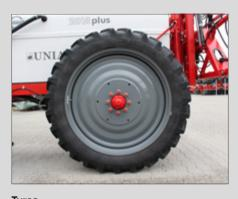
**Tyres** Tyres are one of the crucial factors during work in order to protect soil. In PLUS sprayers it is possible to install tyres of 270/95 R42 size.
