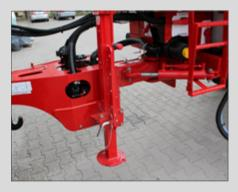
Semi-automatic tracking drawbar enables driving the sprayer along the tractor wheel traces. The trace copying is possible due to two sensors and a chain mechanism.
