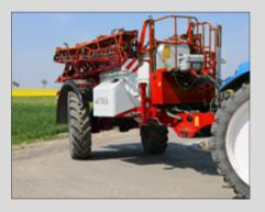
Automatically controlled turnable axle It ensures precise sprayer tracking along the tractor wheels.
