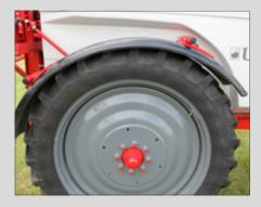
Mudguards They provide the protection of the sprayer control elements against dirt, adjusted depending on the tyre size.
