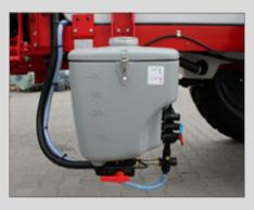
**Diluter** Diluter of 45 I capacity for thinning the materials used for the plant protection, equipped with two nozzles for precise washing working liquid from hopper walls and a nozzle for packaging washing.
