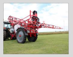
Independent beam The application of such a beam largely facilitates spraying on the fields with numerous obstacles (posts, trees).
