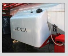
Two hoppers located symmetrically on the machine sides For clean water, 300-litre capacity each, ensure even sprayer load distribution and lower the machine centre of gravity.
