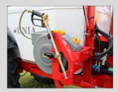
**External washer** It is safe and easy device for the operator and the natural environment used for washing of the sprayer directly at the field.
