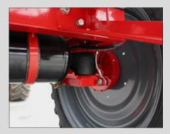
**Mechanical axle shock absorption** It improves driving comfort and extends the lifetime of the sprayer. The vibration transferred to the structure of the entire sprayer during the field work and transport is largely reduced.
