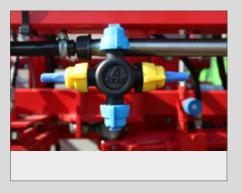
**Optional equipment** 4-position heads with a set of sprayers available as an option.
