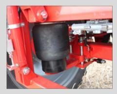
Pneumatic axle shock absorption Installed in a standard option, highly improves driving comfort and extends the lifetime of the sprayer. The vibration transferred to the structure of the entire sprayer during the field work and transport is largely reduced.
