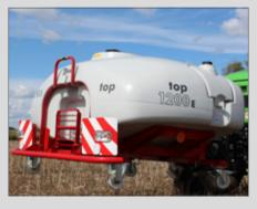
Front tank TOP 1200 It enables increasing the LUX and REX capacity up to 2400 l. Hydraulic or electric pump drive available.
