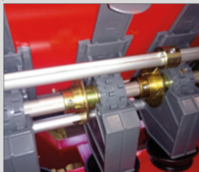
The seed dispensing system comprises of two metering rollers for sowing fine seeds (rape) or large seeds (pea), that precisely collect the seeds from the bottom flaps.
