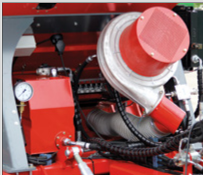
The fan is powered by a hydraulic motor of the output of 24 l/min.
