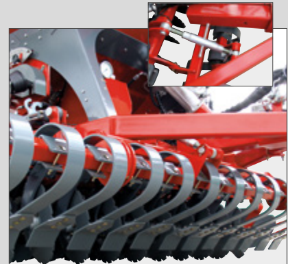
Front levelling spring board design evenly levels the surface of soil before the cultivating discs, which facilitates pre-sowing soil compaction. Easy adjustment of operating pitch with bottle screws.
