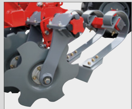
Cultivation discs of the diameter of 460 mm are mounted on a leg and protected with rubber shock absorbers. Mounted maintenance-free bearings ensure comfortable work.
