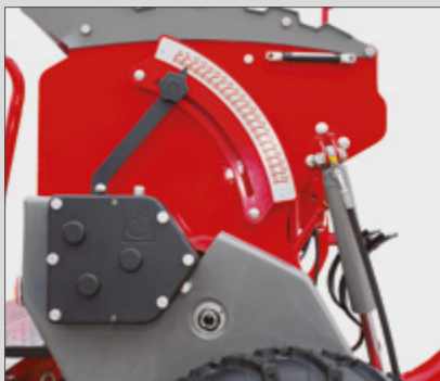
Precise, individually tested transmission gear each ensures accurate sowing pattern.
