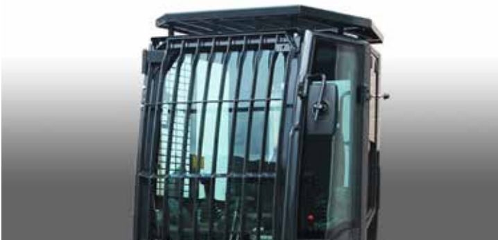
Additional front and rear protective grills with FOPS level II certification
