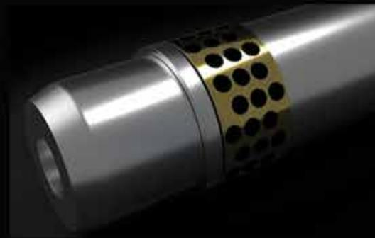
Bronze-graphite bushings used in boom-arm and boom-frame connection points increase the lubrication period, and greatly prevent the wear of the pins because of graphite, having a very high grease absorption and retention capability, embedded in the inner structure of the bushings.
