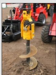
Earth drill installation
