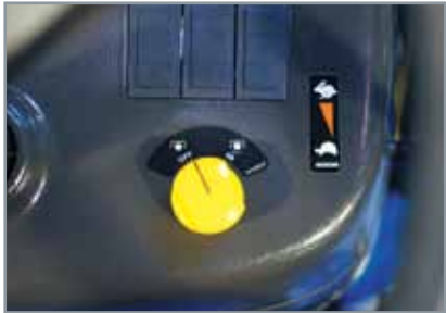
Independent PTO Independent PTO easily operated by switch on the dashboard
