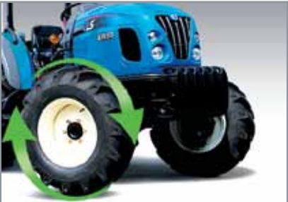
Quick turn (Optional) The quick turn function minimizes the turning radius and offers superb performance, particularly in narrow places
