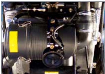
Large capacity Air cleaner This not only has a higher air purification capacity, it also makes maintenance easier thanks to the longer filter use period
