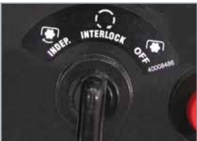
Standard Independent PTO Easy PTO on/off Control for a variety of works
