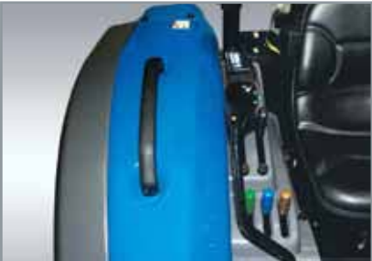
Fender Expansions Fender extensions protect the operators from mud splashes and Large handles are equipped on both sides for easy mounting and dismounting.
