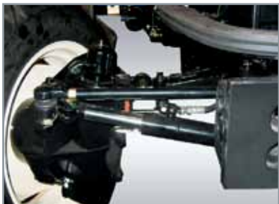
Water proof Front Axle Water and rust proof front axle features a strong structure and durability. It offers the best performance in paddy fields
