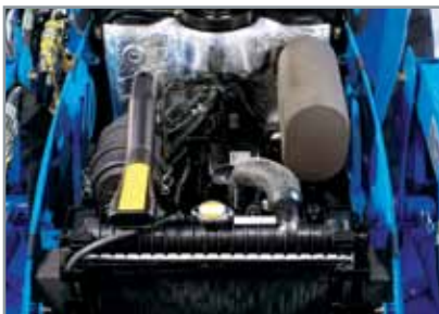
Tier 4 interim engine(Mitsubishi) Eco-friendly, fuel efficient engine delivers quiet, reliable performance. Rubber engine mounts reduce operator platform vibration
