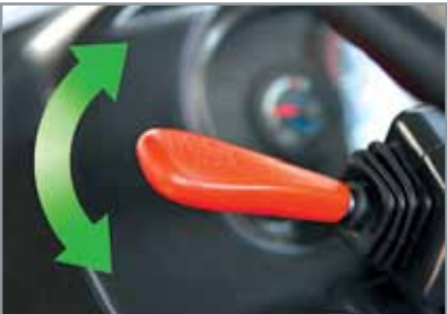
EZ-shift (Optional) Repeated go Forward and Reverse work can be done using only your fingertip. It uses Electro-power, which minimizes engine power loss
