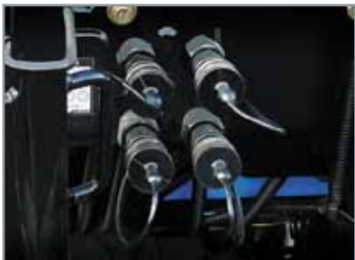
Remote control valve Max 2 pairs of remote control valves offer high compatibility with various implements
