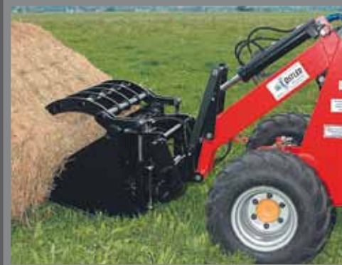
Thanks to the tool holding fixture, which meets the DGS Euro standard, commercially available tools can be used.
