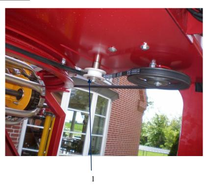
Tension the belt by shifting the tensioning wheel (1)
