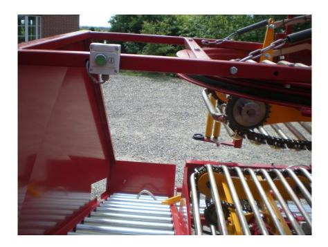
Turn the rotor using button (1).
