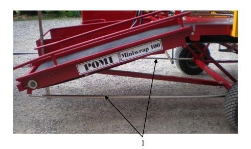
When installing the wrapper on the baler, it is important to ensure as high a pressure on the baler as possible, preferably so the bales start to glide up as soon as they run off the baler. This ensures the smallest possible pitch on the belt and prevents the bales from stacking up.
