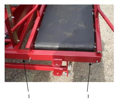
Adjust the belt sideways by slackening the bearings; next adjust the two screws so the belt runs across the middle of the rollers.
