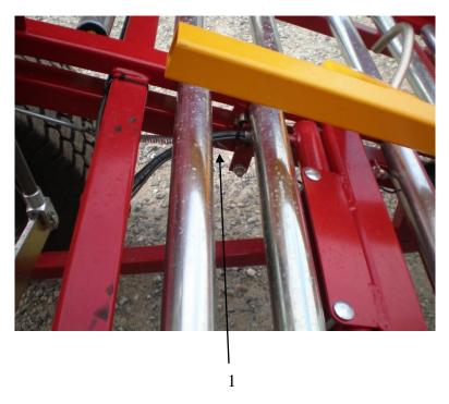
Adjust the sensitivity of the bale sensor by shifting the plate (1).
