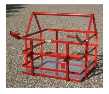
The basket can take approx. 15 rolls and 1 roll of end plastic Inner measure:  $1000 \times 1100 \text{ mm}$  - High = 620 mm
