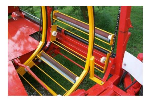
With the help of the front loader, raise the unit above the rear-door and put it down on place, screwing it fast. Move the hoses from the machines' oil motor to the round bales' equipment. Mount the spear, the support plate and the steering brackets on again.
