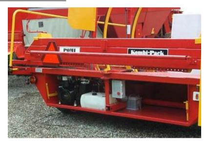
Consist of 2 holders placed on the pushing bar giving space to a roll of film in between. The film is carried under the pushing bar, over the support plate, the rolls and the rear-door.
