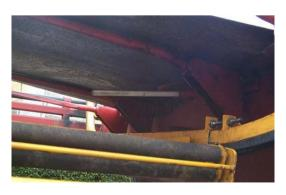
A film guard is placed under the support plate; it is consisting of a bar, which is touching the wrapped film at the place where there is only one lay. If the film brakes, the bar will fall down, activating a contact, which stops the machine. The machine re-starts with one pressure on the remote control, keeping the finger on the button until the film guard is in contact with the film.
