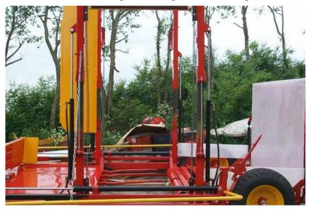
8 bolts are necessary to fix the chains when sinking the frame. Get the stretching rollers into the position shown on the below picture. Fix the 4 bolts at the bottom. Pull the frame down and fix the 4 bolts at the top.
