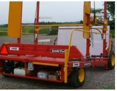
The equipment for silage is composed of 2 bars as shown on the picture. They can be mounted at two different highs on the frame. The winding chain is placed above the bars and it is shorted to give the same length to the 3 chains.
