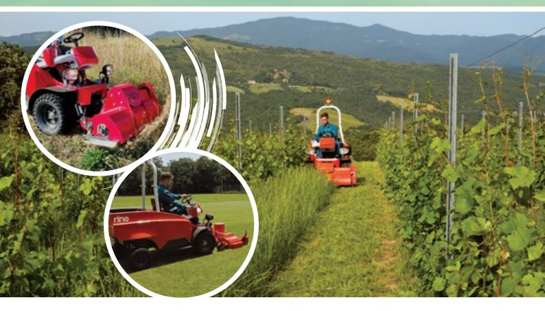
**RINO**<sup>®</sup> offers the most singular driving experience of any tractor of its kind. It has an unbeatable acoustic level, a comfortable driving position with full 360° visibility, front wheel drive and two rear wheels for steering with an optimal turning radius for easy manoeuvrability in tight areas. The front mounted implements provide a perfect and complete view of the working area allowing quick and safe intervention by the operator.
