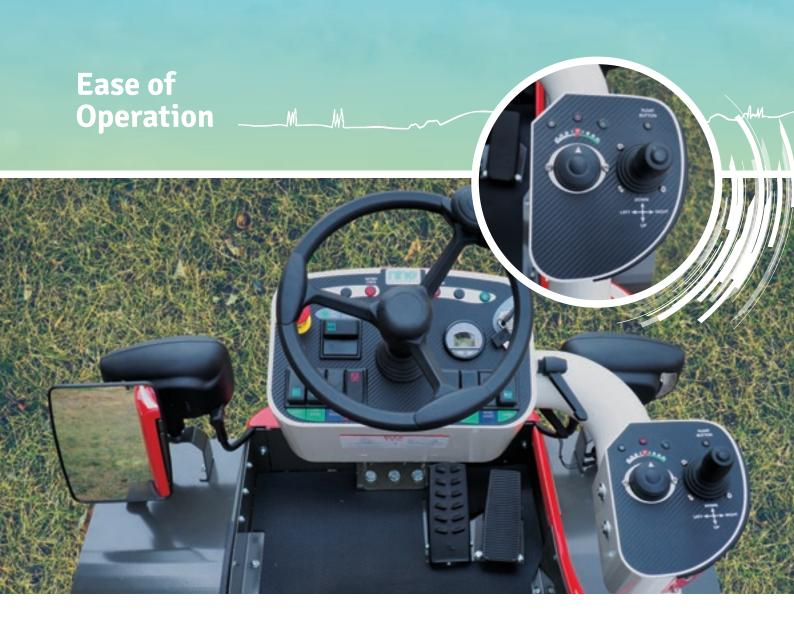
The control and information centre of the **RINO**<sup>®</sup> is designed for functionality with only essential elements. The principal data is shown on a display with the possibility to select the data required. The direction of travel and maximum speed are regulated by a rotary dial.
