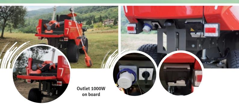
**RINO**<sup>®</sup> provides a "real" 18 kW (24cv) to two equal size electric motors, one to power the tractor and one to power the implements. It can be used with many power-hungry implements such as chippers, snow turbines, helicoidal lawn mowers.
