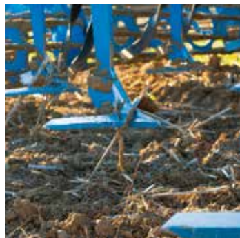
Gåsefodsskær, placeret med overlap
