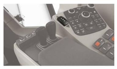
The **TIPSHIFT** function provides operator ease of operation. It is possible to change the direction quickly by pressing a single key without using the gear lever when the machine is moving forward or backward while taking under the load or unloading. This increases productivity and ensures safe operation without the loss of steering control.
