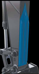
Reinforced arm supporting parts
