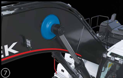
Reinforced boom cylinder cast bearing
