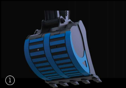
More durable anti-wearing plates (Hardox 450 HB)
