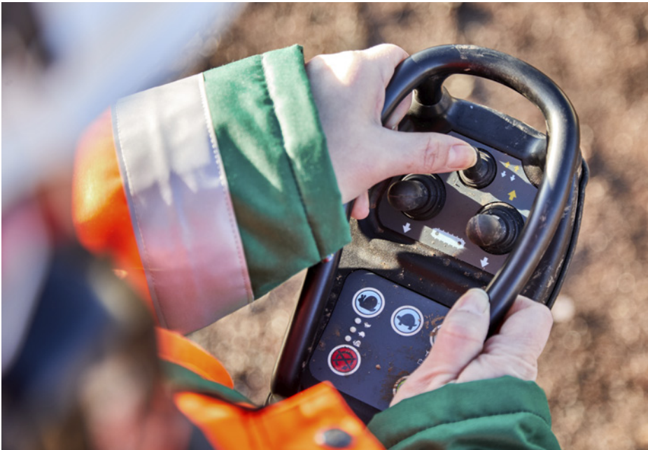
Remote controller for crawler tracks as standard.
