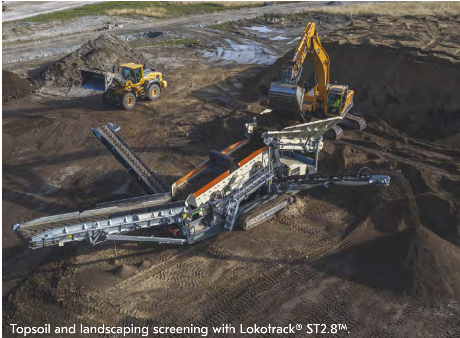
Screening sand and gravel with Lokotrack® ST2.8™.
