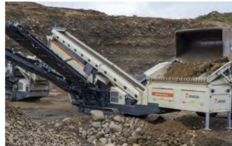
Large feed box allows closed circuit process.
