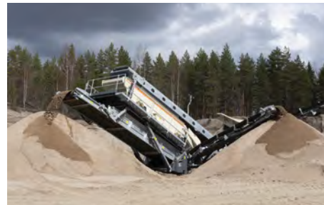
Adjustable conveyors for high stockpiles.
