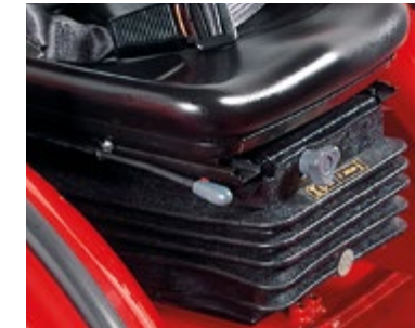
PNEUMATIC SEAT Latest generation with air springs.
