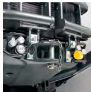
QUICK COUPLERS Front lift > 6 rear couplings.
