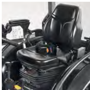
PNEUMATIC SEAT Latest generation air suspension seat.
