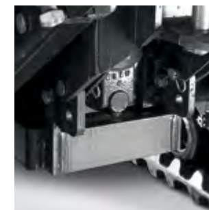
BALANCING BALLAST Supplementary ballast for optimising vehicle balance.
