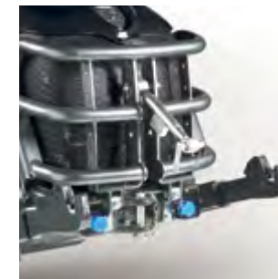
FRONT LIFT Used together with the bullbar, it allows all the frontal equipment to be used with multiple hydraulic connectors.
