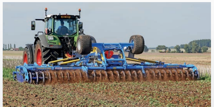
Side frames with hydraulic pressure perfectly follow uneven terrain
