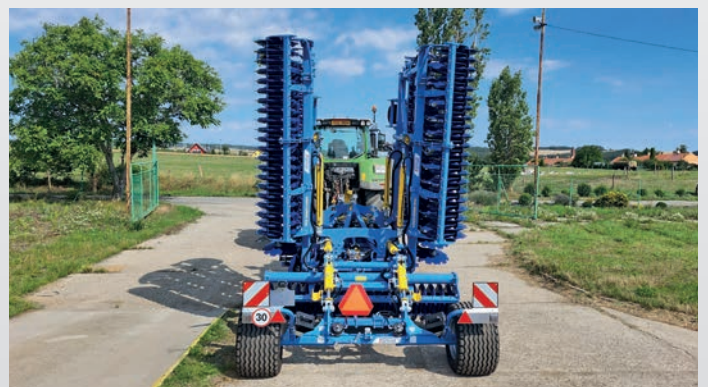
Transport dimensions: width 3 m, height 4 m
