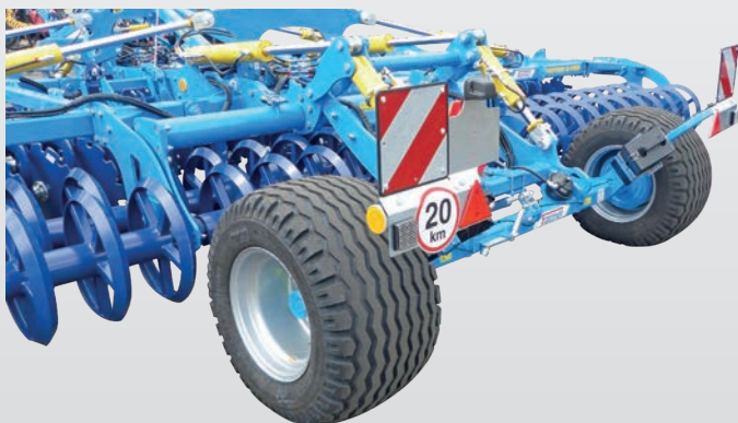
Massive transport axle with brakes
